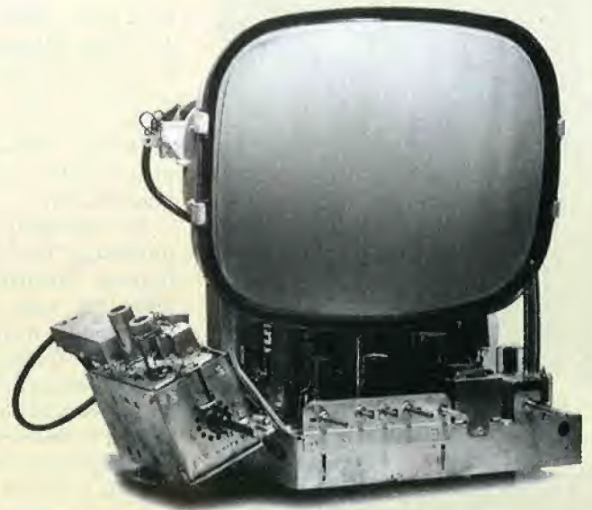
An early AWA chassis with turret tuner on side. The first Australian TV picture tubes had very rounded screen and edges, so advertisers proclaimed it was 'to see the image from a wide angle'. Later when screens were flat, the same was claimed, plus 'for minimum reflections'.
