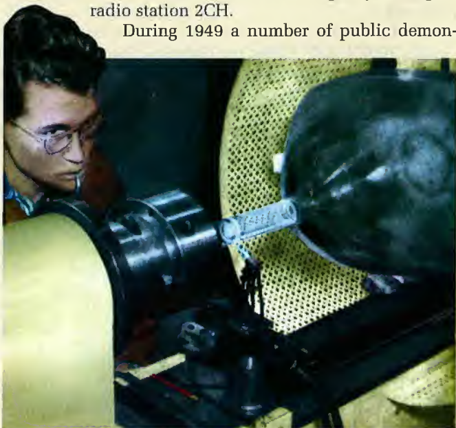
In June 1956, before regular broadcasts, this AWW pilot production run was demonstrated to 'Radio TV and Hobbies' . The operator is using a tube in his mouth to control the flame, part of the process called 'kinescope blowing'.
